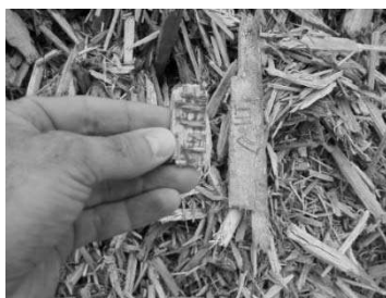
Figure 5 Rough grind mulch contaminated with colored plywood
